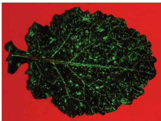
Fluorescent particle coverage of canola leaf (three- to five-leaf stage) showing fungicide deposition achieved at this growth stage. (Photograph: Gideon van Zyl)
